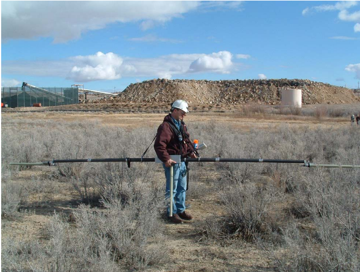
Gradiometer receiver at first survey area. Depth of cover over the entries is approximately 80 to 100 Feet.
