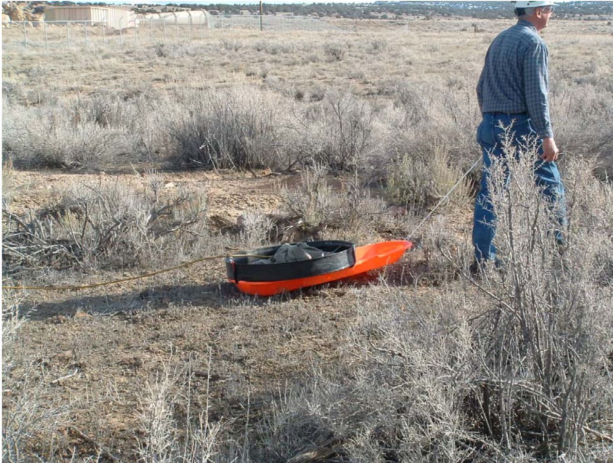
Pulling the mobile transmitter parallel to the receiver survey line.
